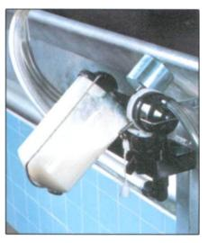
**3.** Canister tips down as milk weight increases. Second letdowns are handled during this automatic phase.
