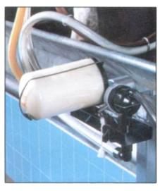
**4.** Milk flow decreases to the take off time you preset. Counterweight pivots canister up to off position
