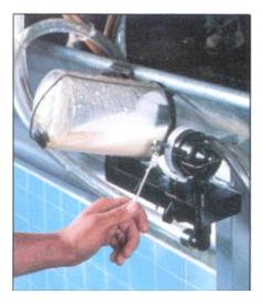
**1.** Milker pulls "trip" cord which sets valve in "milk" position releasing cylinder vacuum to allow claw attachment
