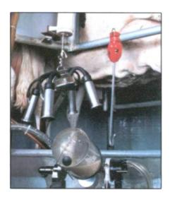
**6.** Cow is milked out. Vacuum is on at cylinder, claw is retracted. Detacher is ready for next cow.
